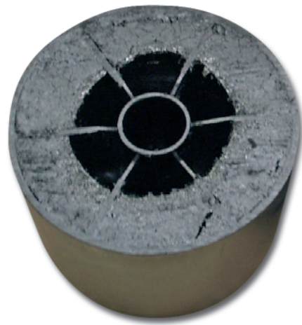
Sectioned Rotor with Contaminant
