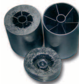
Sectioned rotor full with contaminant. Section rotor displaying the internal ribs.
